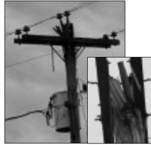
Lightning struck and split the top of a power pole just 40 feet from where services were about to be held in Missouri. Services and a dinner/dance were unaffected
